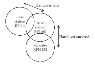
Also, a handset must never be able to detect two radio units (base stations or repeaters) with the same RPN at the same time. The handset will not be able to make a handover. If an RPN is reused, the units must be placed at a fair distance from each other.
