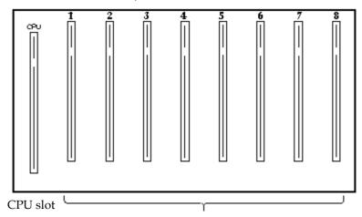
Extension card slots (8 for Spectralink DECT Server 8000, 3 for Spectralink DECT Server 2500)
