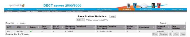
3 If you only want to display the base stations that are connected, select **Show only connected RFP's** check-box and click the **Refresh** button.
