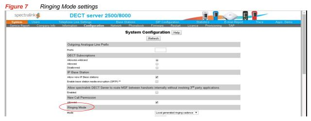
2 On the **Ringing Mode** section, from the **Mode** drop-down list select one of the following options: **Ringing cadence follows (I)PBX** or **Local generated ringing cadence**.
