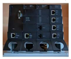
Figure 4 Spectralink DECT Server 2500 Chassis with CPU (with Link option) and Interface cards
